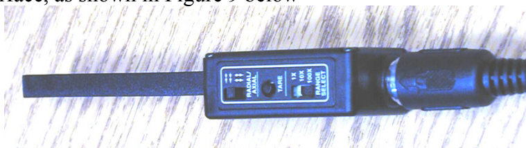
Figure 8 Top view of the magnetic field sensor, showing (from right to left) the RANGE SELECT switch, the TARE button, and the RADIAL/AXIAL switch, which is set to RADIAL.
