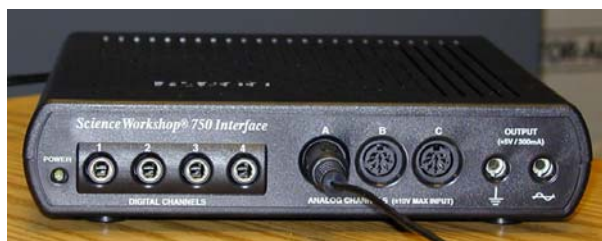
Figure 9 Frontal view of the 750 Interface, with the magnetic field sensor plugged into the “A” analog channel port.
