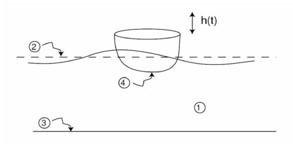
Figure 2.1. Boundary conditions for the total potential must be met at three places: sea floor (3), free surface (2), structure surface (4). The continuity equation must be satisfied within the fluid (1).
