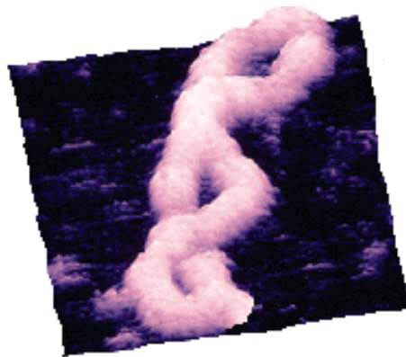
The high resolution of the SPM is able to discern very subtle features such as these two linear dsDNA molecules overlapping each other. 155nm scan.
