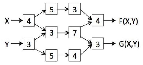
(A) Using ideal zero-delay registers, mark the location of the minimal number of registers necessary to achieve maximum throughput. Give the latency and throughput of your pipelined circuit.
