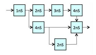
(B) (2 points). Show the maximum-throughput 2-stage pipeline using a minimal number of registers.
