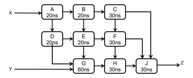
Although you don't know the function of each of the component modules, they are each combinational and marked with their respective propagation delays. You have been hired to analyze and improve the performance of this device.
