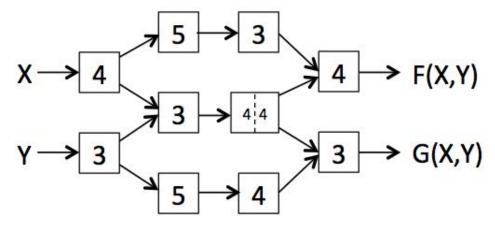
(B) Using ideal zero-delay registers, mark the location of the minimal number of registers necessary to achieve maximum throughput. Give the latency and throughput of your pipelined circuit.
