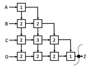
(A) Please pipeline the circuit above for maximum throughput with the minimum possible latency using ideal pipeline registers ( $t_{PD} = 0$ ,  $t_{SETUP} = 0$ ). Show the location of pipeline registers in the diagram above using filled-in circles, like the one shown on the Z output. Please give the latency and throughput of the resulting pipelined circuit.
