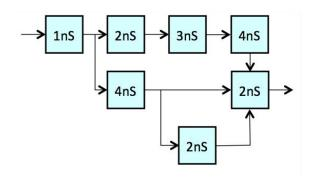
(D) (2 points). Show the maximum-throughput 4-stage pipeline using a minimal number of registers.
