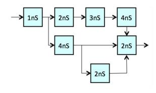
(C) (2 points). Show the maximum-throughput 3-stage pipeline using a minimal number of registers.
