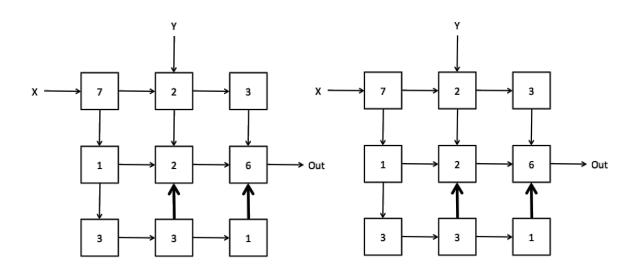
(C) You are now asked to consider the performance of this circuit using different clock periods while achieving the minimum latency. For each suggested t<sub>CLK</sub>, specify whether or not you can create a **valid** pipelined circuit using that clock period. If you can, then provide the latency and throughput of the resulting circuit and specify the number of registers at each input. If it results in an invalid pipeline, enter NA for the rest of the row.
