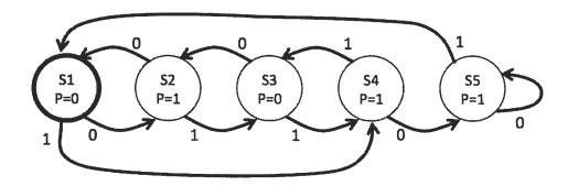
(A) (1 Point) The FSM has been processing inputs for a while and we would like to determine its current state. After entering three additional inputs "000", we observe that we have reached a state where P=0. Please circle the possible values for the state *before* the additional three inputs were entered.
