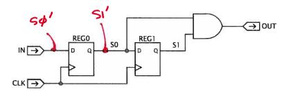
Please describe the operation of the FSM by filling in both the state transition diagram and the truth table shown below. The two-digit state names in the state transition diagram are S0,S1, the logic values present at the outputs of REG0 and REG1 after the rising edge of the clock. In the truth table, S0' and S1' are the values that will loaded into REG0 and REG1 at the next rising clock edge.
