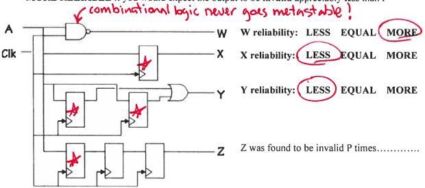
These registers are particularly susceptible to metastability since they are connected to input A.
