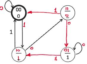
(C) If this FSM is implemented using a 2-bit state register and a ROM, what size ROM would be needed? Please specify the number of locations (entries) of the ROM, and the width of each entry.
