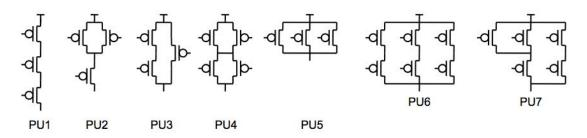
The web site explains that the customer can choose which inputs are connected to each PFET, allowing their pullups to be used in various ways to build gates with various numbers of inputs. Since Pullups Galore charges by transistor, you are interested in selecting pullups using the minimum number of transistors for each of the 3-input gates you are designing.
