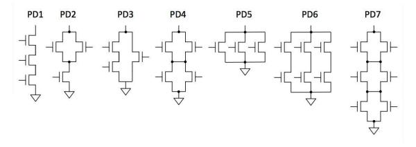
The web site explains that the customer can choose which inputs or constants (GND, VDD) are connected to each NFET, allowing their pulldowns to be used in various ways to build gates with various numbers of inputs. Since Pulldowns-R-Us charges by transistor, you are interested in selecting pulldowns using the minimum number of transistors for each of the 3-input gates you are designing.
