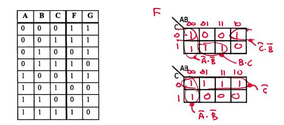
Give the **minimal sum of products** (minimal SOP) logic equation for each of the two functions. Then determine if the minimum sum of products expression would result in a **lenient** implementation of the function. If it does, then enter "**SAME**" for the lenient SOP expression. **If not**, specify what sum of products expression would result in a lenient implementation. Hint: Use Karnaugh maps above to determine the minimal sum of products.
