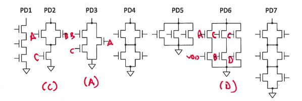
The web site explains that the customer can choose which inputs or constants (GND, VDD) are connected to each NFET, allowing their pulldowns to be used in various ways to build gates with various numbers of inputs. Since Pulldowns-R-Us charges by transistor, you are interested in selecting pulldowns using the minimum number of transistors for each of the 3-input gates you are designing.
