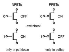
We want *complementary* pullup and pulldown logic, i.e., the pulldown should be "on" when the pullup is "off" and vice versa.
