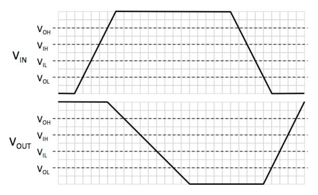
(A) Based on the figure below, what is an appropriate choice for the contamination delay of the gate?
