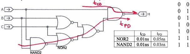
(A) Using the timing specifications shown above for NOR2 and NAND2, compute the contamination and propagation delay for the implementation of H shown above.
