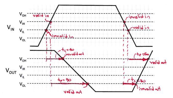
(A) Based on the figure below, what is an appropriate choice for the contamination delay of the gate?
