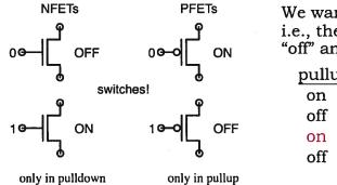
We want *complementary* pullup and pulldown logic, i.e., the pulldown should be "on" when the pullup is "off" and vice versa.
