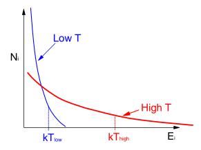
At room temperature (300 K),  $k_BT/hc = 208 \text{ cm}^{-1}$ . This means that energy states near or below 200 cm<sup>-1</sup> will have thermal population at room temperature. These are typically only rotational states in the ground vibrational and ground electronic state.
