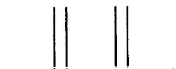
Doublet of Doublets (1H) Proton coupled to two non-equivalent protons which are attached to the same or different atoms
