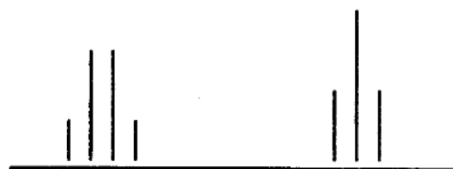
Quartet (2H) and Triplet (3H) Ethyl group \text{CH}_3\text{CH}_2\text{-Z} Z = non H-bearing atom, typically O, N, C of Ar, etc.
