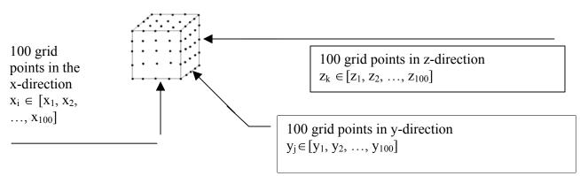
The total number of grid points (x<sub>i</sub>, y<sub>j</sub>, z<sub>k</sub>) in the 3-D mesh is  $10^2 \times 10^2 \times 10^2 = 10^6$
